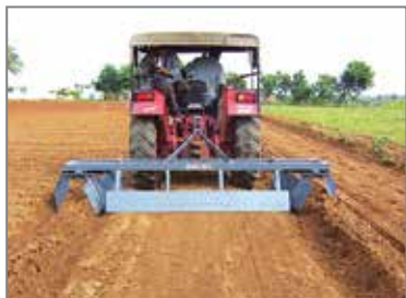
Levelling the field with a leveller
